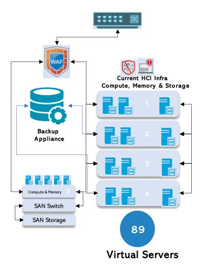
**DC Network:** The schematic depicts the Core Switches in HA mode. Connectivity of the Converged and Hyper-converged Server infrastructure to the rest of the Network at HO is depicted along with Web Application Firewall (WAF).
