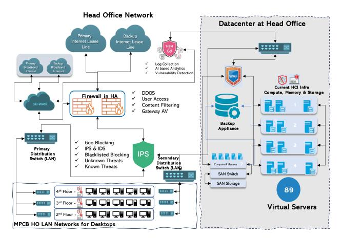
MPCB network gateway is protected with NGFW in HA. The firewalls act as single gateway for LAN, DMZ, SDWAN and WAN environment. The entire traffic passes through the gateway firewall.
