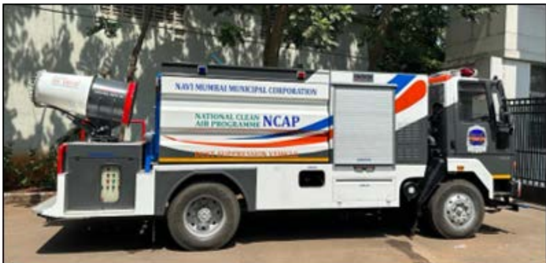
Dust Suppression Vehicles with Multi-Purpose Sprayer
