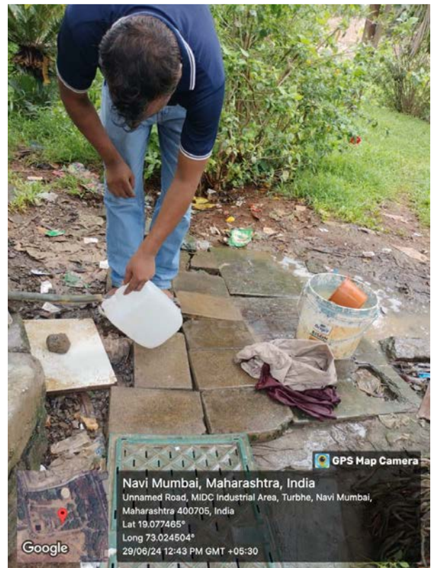
Groundwater Sampling – Navi Mumbai MSW Dumping Ground Borewell Water Turbhe
