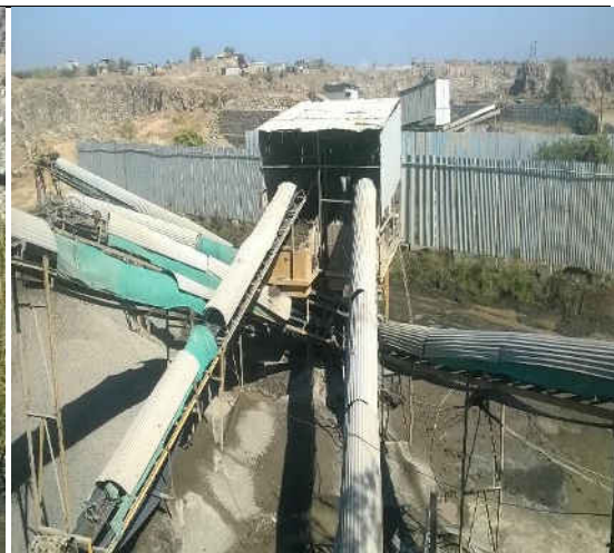
Photograph-2. Covered conveyor belts and partially covered vibratory screens.
