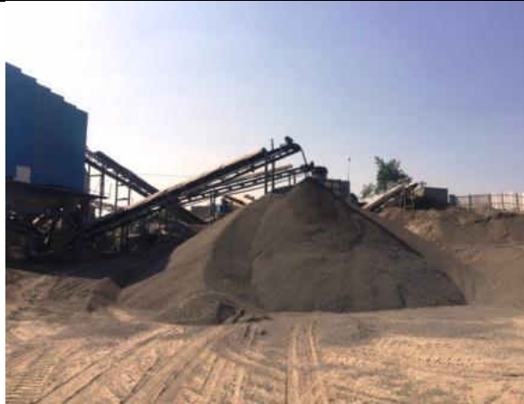
Photograph: The heaps not covered by the present sprinkling system
