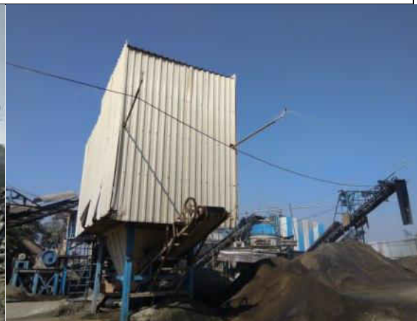
Photograph: Sprinklers for stored material and closed screen house
