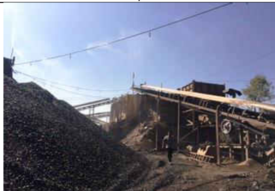
Photograph: Sprinklers fixed on PVC pipeline overhead
