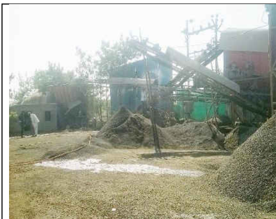
Photograph-1. Sprinklers mounted at conveyor belt nodes, partially covered conveyor belt and vibratory screen.
