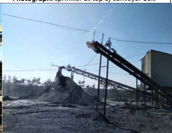
Photograph: sprinkler at top of conveyor belt & fogger system overhead
