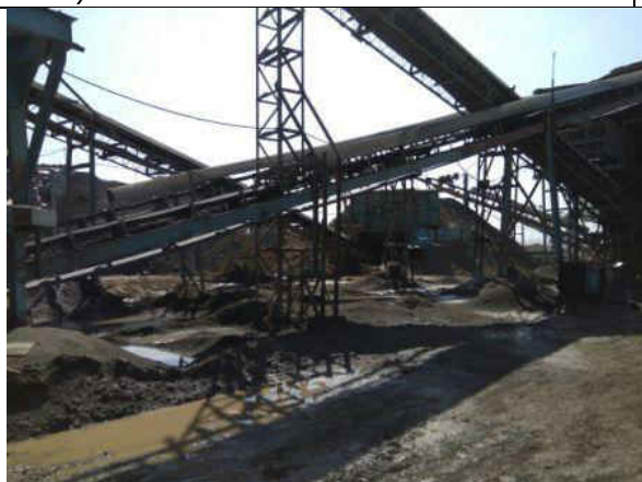
Photograph: Marshy condition due to excess sprinkling & damaged condition of conveyor covers
