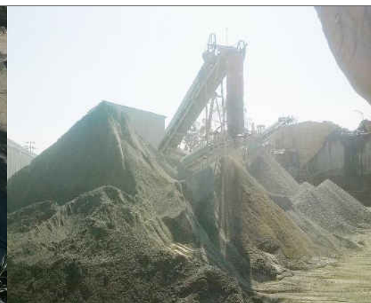
Photograph-4. MS drum used as chute. Product heap height is more than WBW.
