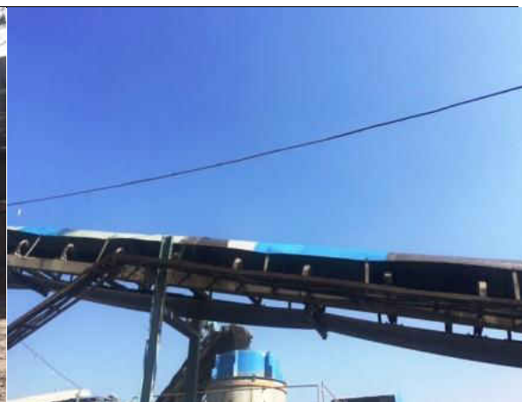
Photograph: Foggers line overhead along the conveyor lines
