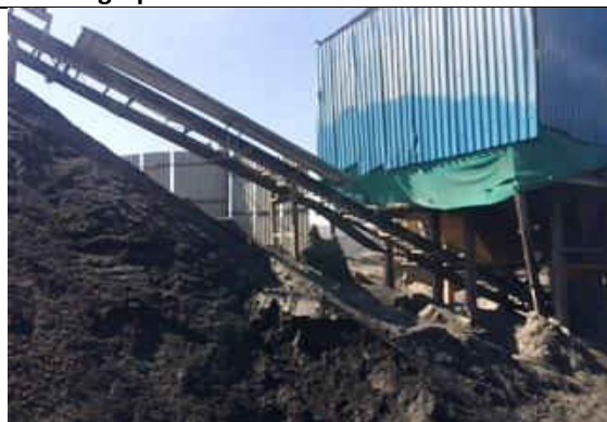
Photograph: The covers of conveyor belts fixed at huge gap above the belt
