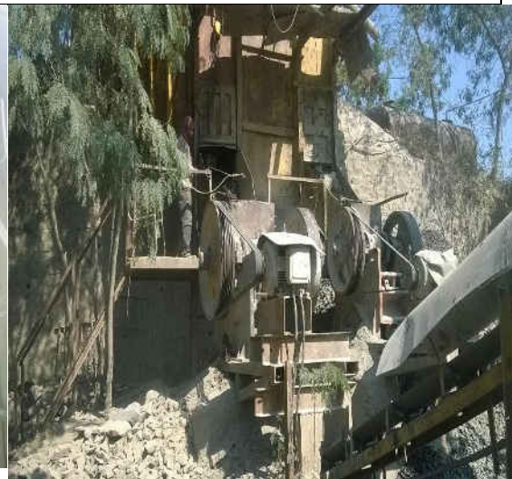
Photograph-4. Person working on Jaw crusher without PPE
