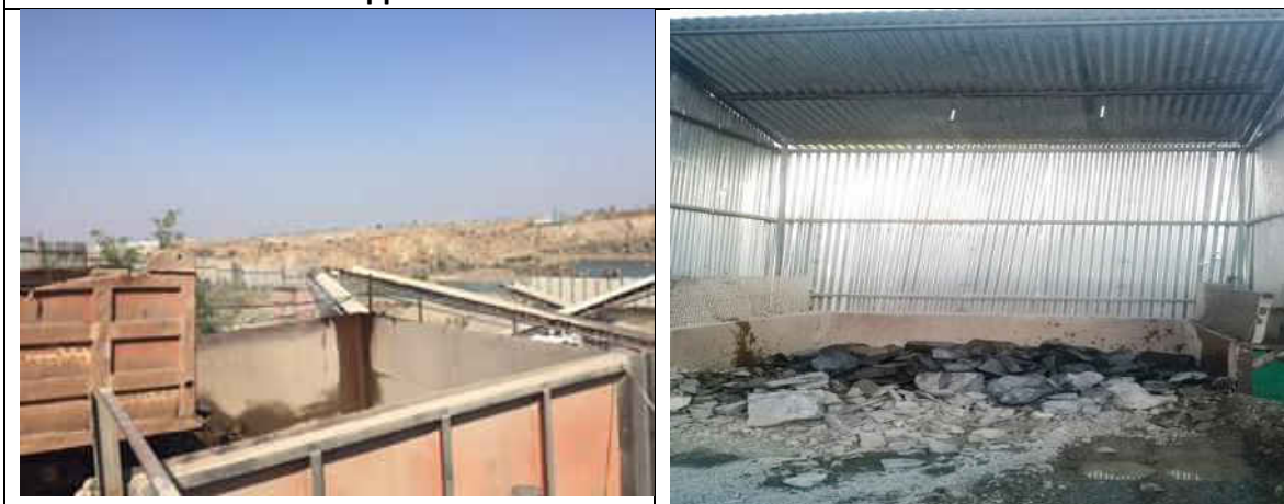
Jaw Crusher Main Hopper without tin shed and with tin shed from three sides and top
