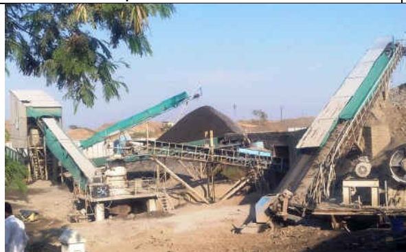
Conveyor belts partly open and partly covered with tin sheets & green cloth. Screen placed in tin sheet housing.
