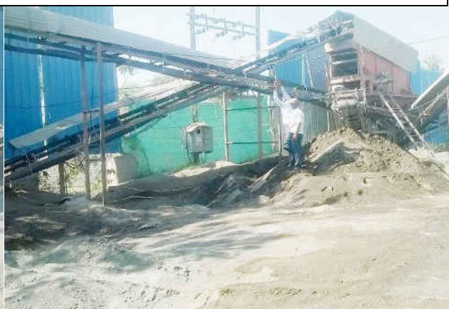
Photograph-4. Gap between conveyor belts and metal cover (jaw crusher to screen).
