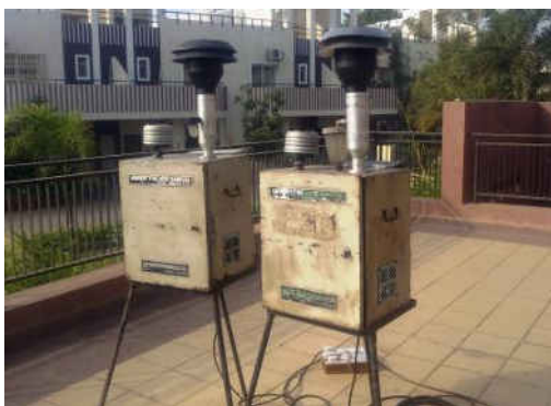
Sampler PEM-ADS 2.5/10 used for Ambient Air Quality monitoring
