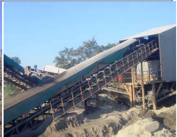
Screen housing covered properly from all sides with front opening. Conveyor belt with enclosure.
