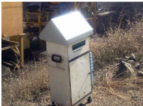
Model: PEM-HVS used for work zone monitoring in Stone Crusher units
