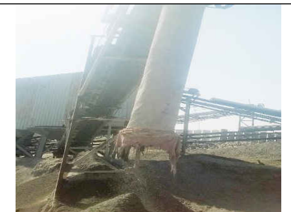
Photograph-5. Metal drums used as chute at crush sand conveyor belt nod (A good practice).
