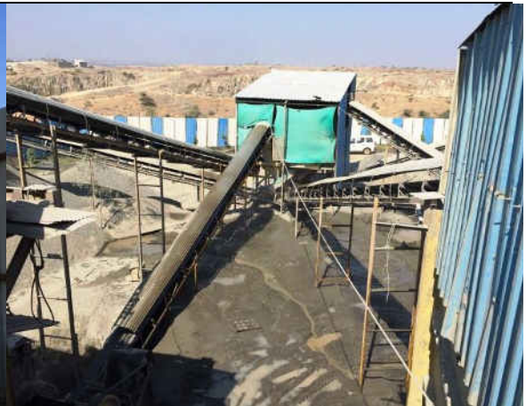
Vibrating Screen housing provided by the unit
