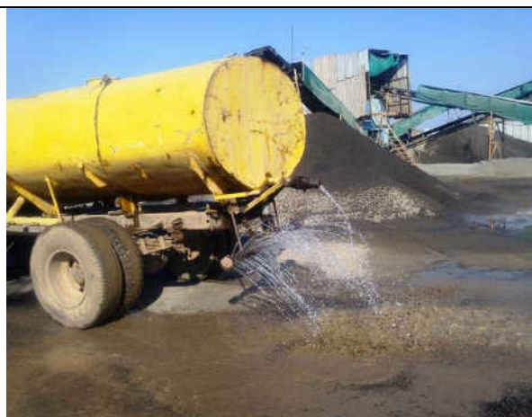
Excessive application of water through tanker in the premises.
