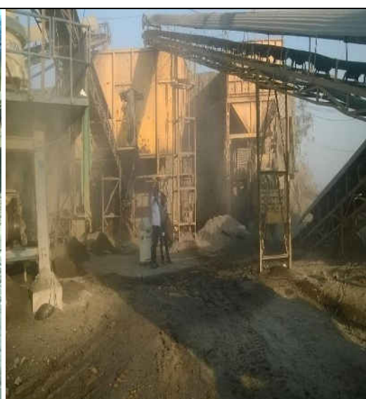
Photograph-4. Emissions from operation of jaw crusher and cone crusher in absence of sprinkling.
