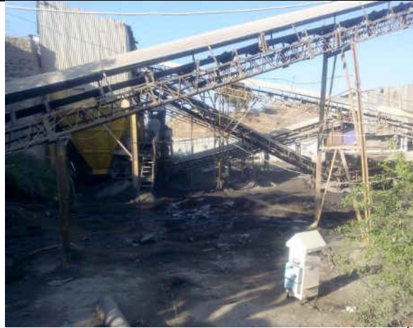
Gaps in sides of conveyor belts. Screen placed in tin sheets housing/shed. Poor housekeeping.
