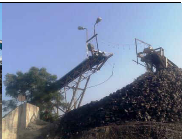
Fogger provided at material transfer points.
