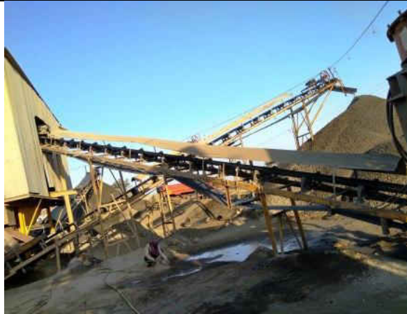
Photograph: Covers of the conveyor belt with more gap
