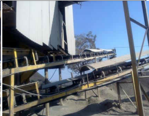
Partial enclosure on conveyor belts and gaps between enclosure & conveyor belts.
