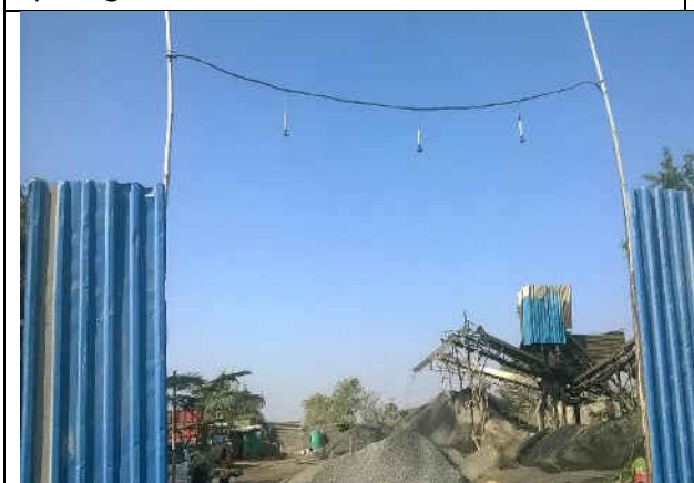
Photograph-3. Water Sprinkling arrangement at gate.
