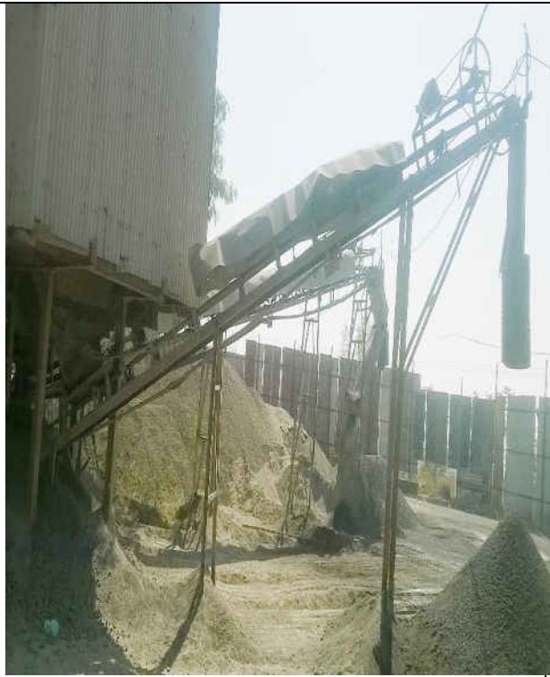
Photograph-1. Sprinklers mounted on conveyor belt and partially covered conveyor belt.
