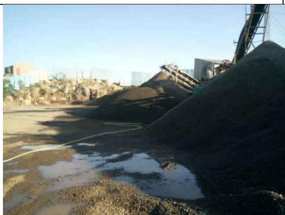
Photograph: sprinkling of water on heaps & ground through flexible hose
