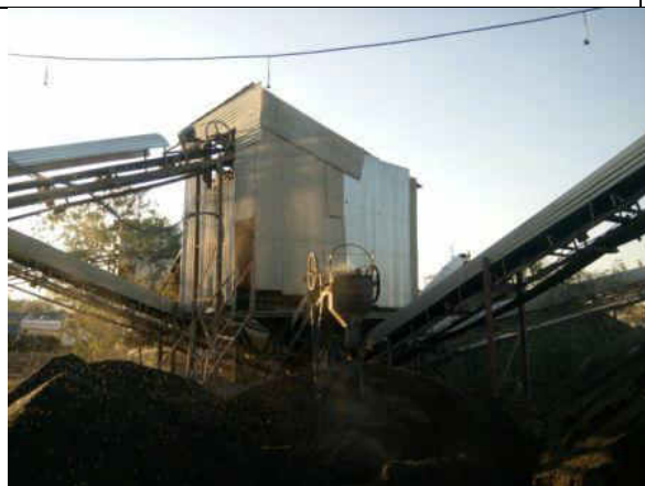
Photograph: sprinklers overhead system and covered screen house
