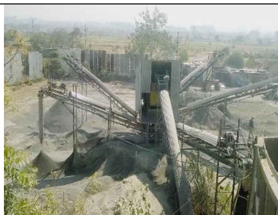
Photograph-6. Vibratory Screen open from conveyor belt entry side.
