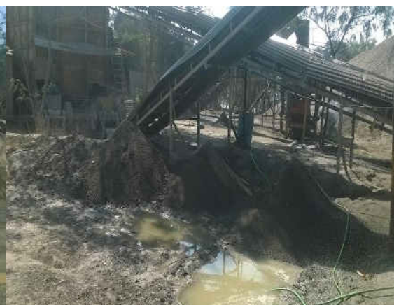
Photograph-4. Spilled material below conveyor belt and water logging due to excess sprinkling of water.
