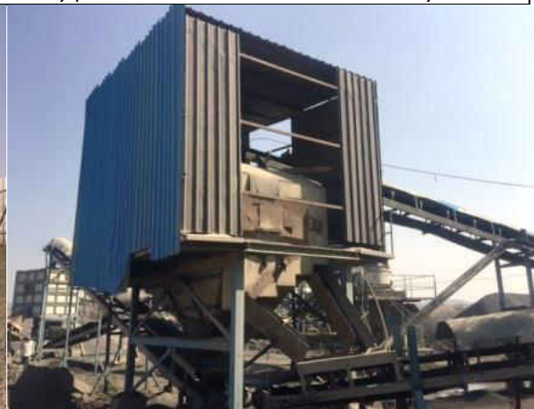
Photograph: Screen housing not covered fully
