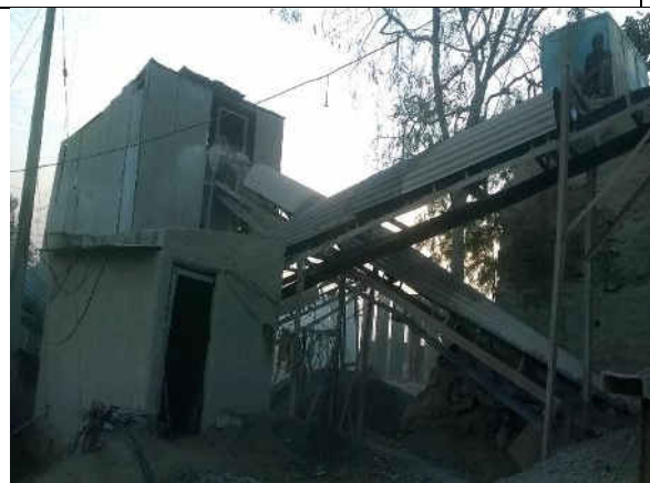
Photograph-3. Vibratory screen enclosed inside a shed which is open at conveyor belt end.
