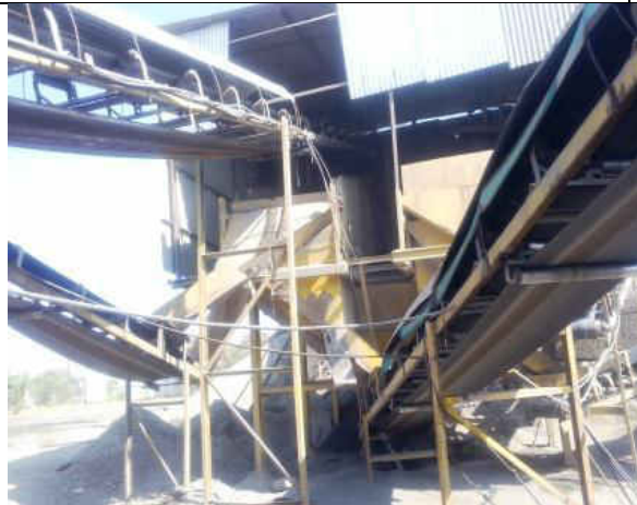
Screen open from top and housing partially covered.
