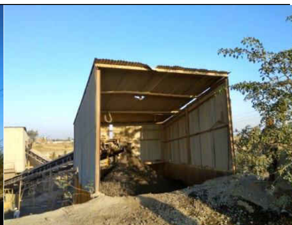
Photograph: Cover for secondary hopper
