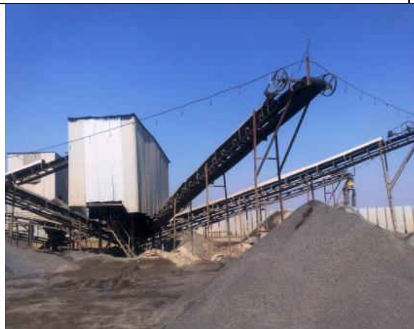
Overhead foggers at material transfer points. Transfer point without chute system and having height more than wind breaking wall. Covered screen housing on backside.
