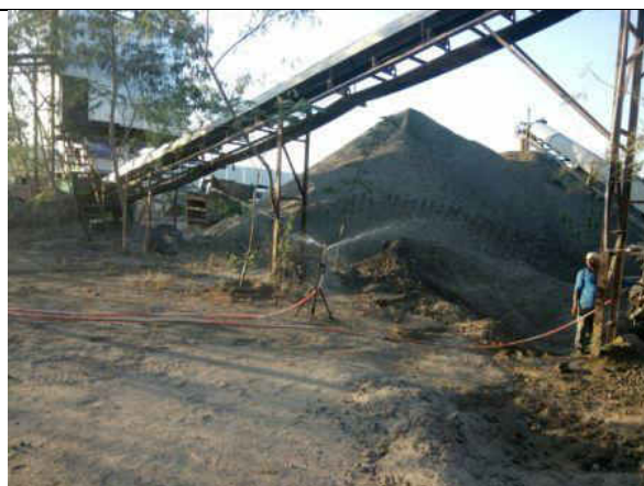
Photograph: movable sprinklers for sprinkling on ground and on the stored material
