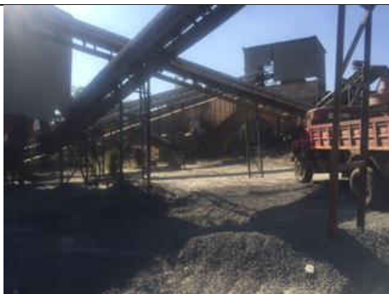
Photograph: The vacant material storage area and covered secondary hopper (non-operational)
