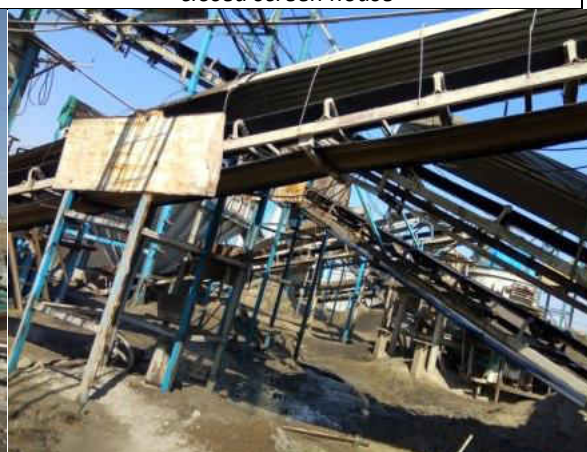
Photograph: Covers of the conveyor belt fixed with more gaps
