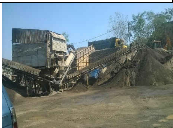
Photograph-3. A view of conveyor belt cover and improperly fabricated vibratory screen shed.
