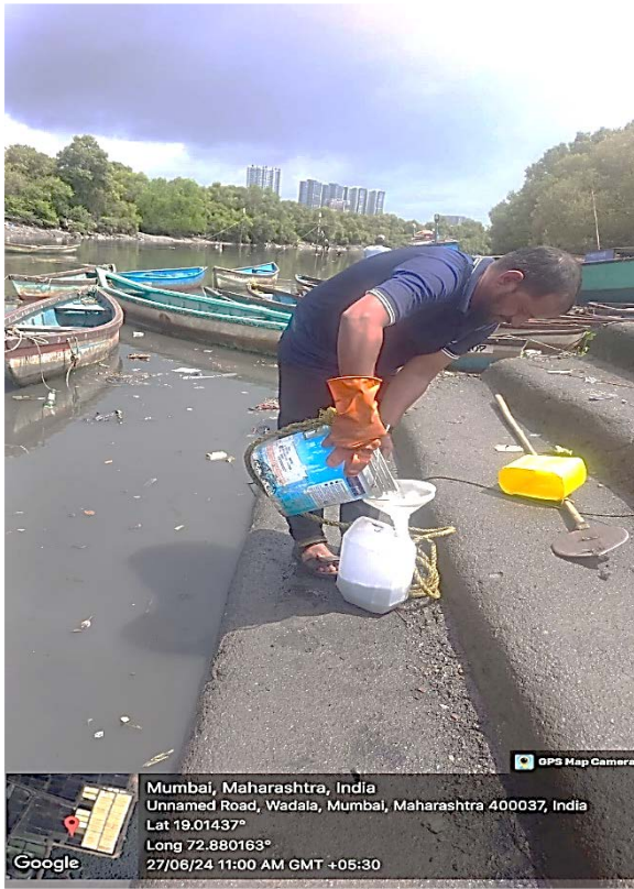
Surface water sampling at Downstream near Mahul Jetty
