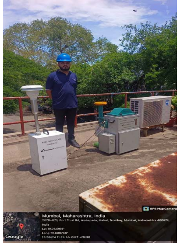
Ambient Air Sampling at Near main gate BPCL
