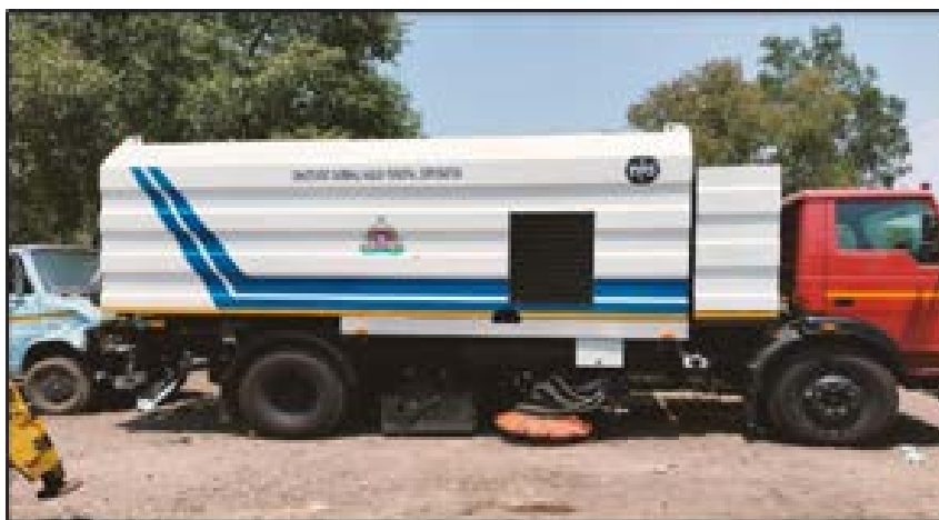
Dust Suppression Vehicles with Multi-Purpose Sprayer-Mechanized Road Sweepers
