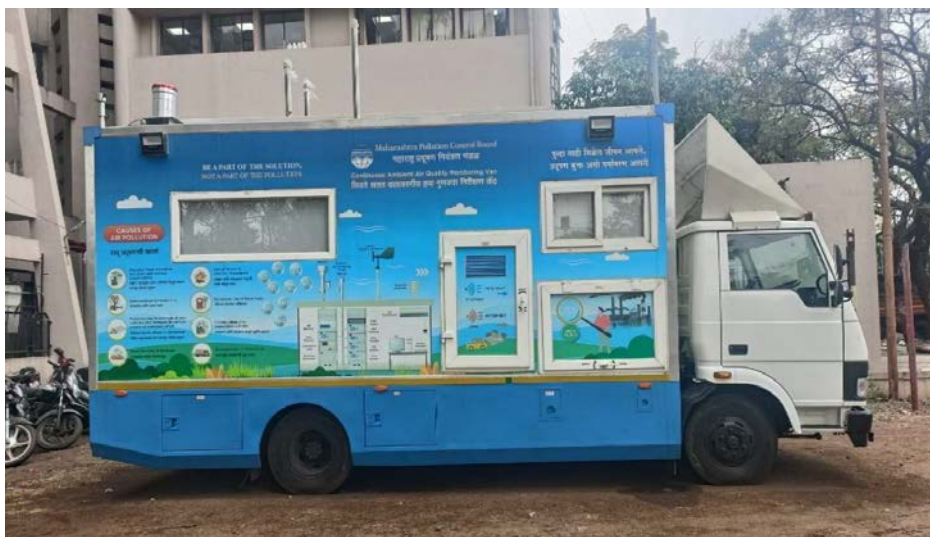
Ambient Air Quality Monitoring (AAQM) Van
