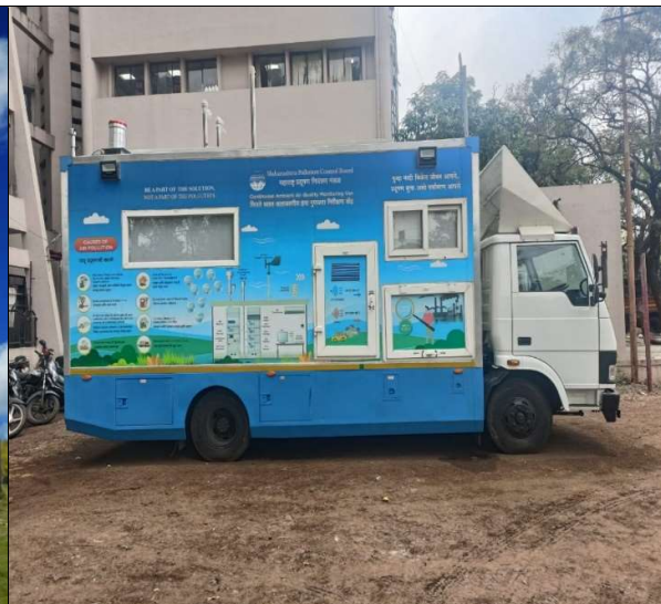
Ambient Air Quality Monitoring (AAQM) Van
