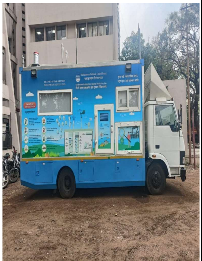
Ambient Air Quality Monitoring Van
