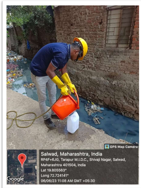
Surface water sampling at Nallah near sump 2
