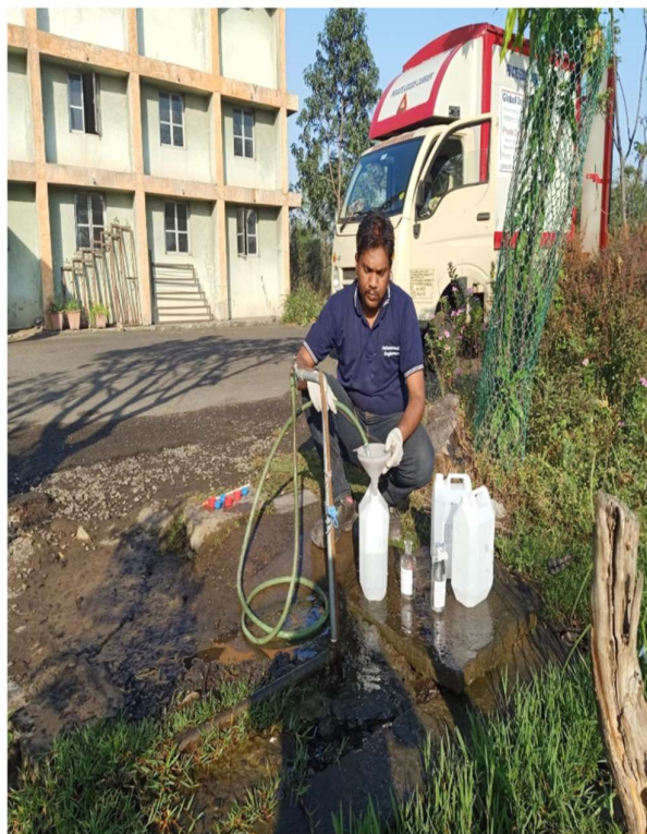
MIDC Tadali – Surface Water Sampling at Raw Water of MIDC WTP
